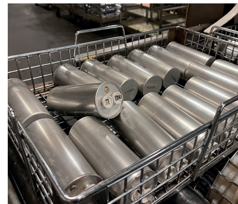
The new water-based system at CD Aero successfully cleans oil from capacitors.
